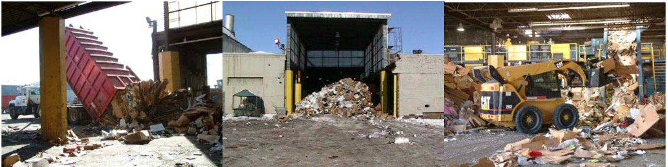
Material gets dumped onto the sorting floor and pushed onto conveyors.
